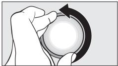
Turn the lamp cover anti-clockwise to remove it. Do not touch halogen lamps with your bare fingers. Use a soft cloth when changing a halogen lamp.
